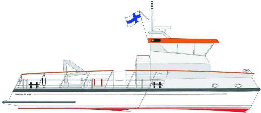
**Mobimar 16 Work offers an exceptionally wide and stable working platform. The vessel hull form is a carefully optimised trimaran. Different load conditions have relatively little influence to speed. Fuel consumption is low allowing for smaller fuel tanks and better payload. Smaller operation costs.**
