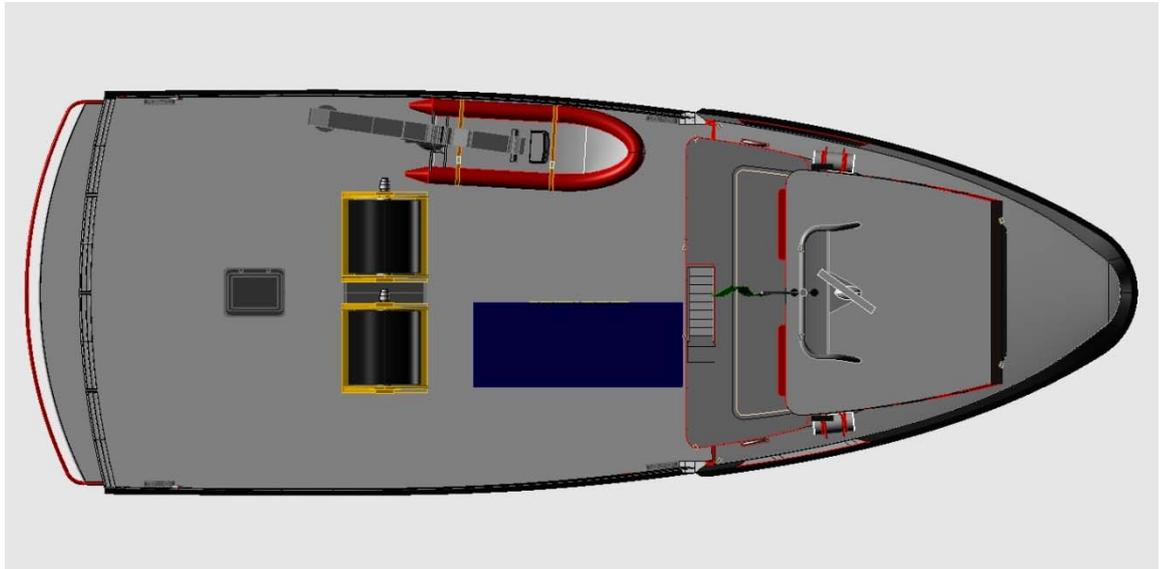
On main deck there is 200 m<sup>2</sup> for Equipment area. This picture shows a 20' container, MOB vessel, two open ocean boom reels 500m of boom on each. There is still a good amount of working space around the deck.
