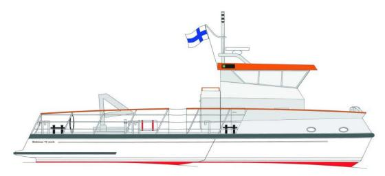
Mobimar 16 Work offers an exceptionally wide and stable working platform. The vessel hull form is a carefully optimised trimaran. Different load conditions have relatively little influence to speed. Fuel consumption is low allowing for smaller fuel tanks and better payload. Smaller operation costs.
