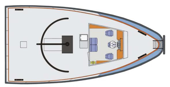
Deckhouse arrangement option No. 2 for tugboat: Control pulpit and additional chairs for navigator and a deckhand. The towing hook has a wide space around with reasonable working area. Aft deck railings are removable in addition.
