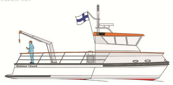
Mobimar 12 Work offers an exceptionally wide and stable working platform. The vessel hull form is a carefully optimised trimaran. Different load conditions have relatively little influence to speed. Fuel consumption is low allowing for smaller fuel tanks and better payload. Smaller operation costs.
