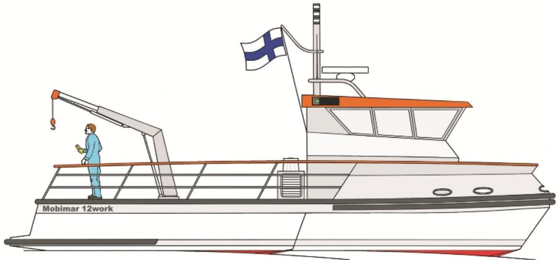
Mobimar 12 Work offers an exceptionally wide and stable working platform. The vessel hull form is a carefully optimised trimaran. Different load conditions have relatively little influence to speed. Fuel consumption is low allowing for smaller fuel tanks and better payload. Smaller operation costs.
