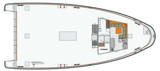
Main deck: Deck house with deck storage for equipment and minor repair works, Mess room with sofas and pantry and cupboards for inventory. Change room for changing the overall and shower and head.
