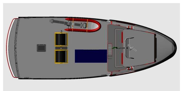
On main deck there is 200 m² for Equipment area. This picture shows a 20`container, MOB vessel, two open ocean boom reels 500m of boom on each. There is still a good amount of working space around the deck.
